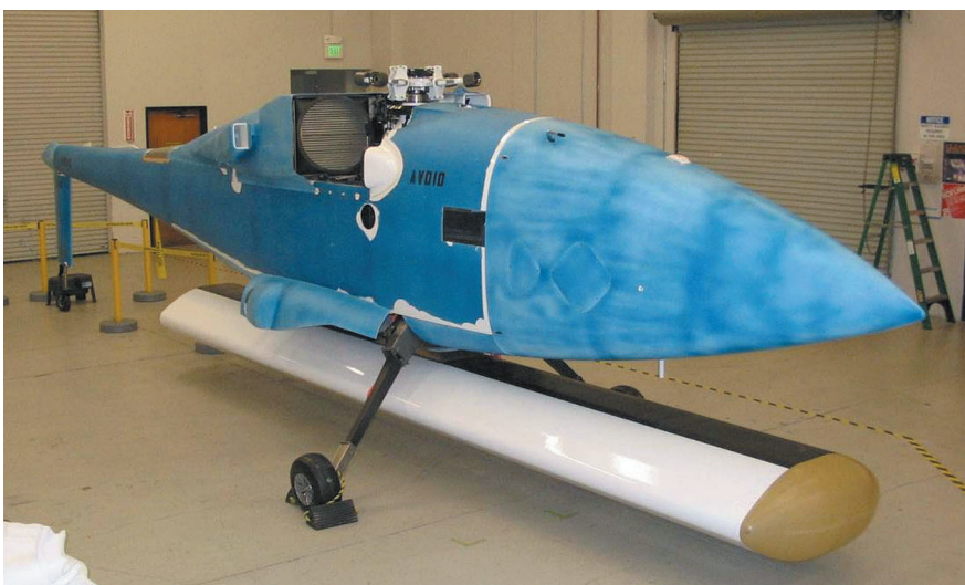
The FORESTER radar system is installed in the A160 Hummingbird aircraft for fit check. Note the sensor's antenna mounted beneath the aircraft. With the landing gear retracted and the aircraft in position over a reconnaissance area, the antenna rotates 90 degrees to a horizontal position to scan a 250-kilometer area every 40 seconds to 50 seconds for hidden enemy soldiers and vehicles.
