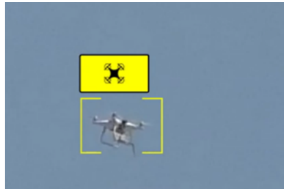
BELOW: Camera using machine intelligence to detect and classify small UAS
