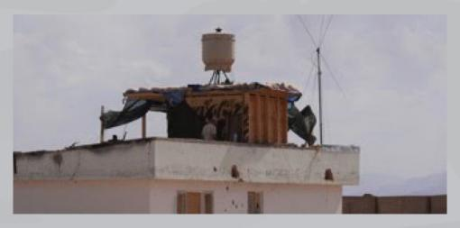
The AN/TPQ-50 radar is a lightweight, compact, L-Band, cylindrical, phased-array radar. It detects, tracks, and classifies traditional aircraft (commercial, small/private, military, and rotary wing) and non-traditional aircraft, such as low altitude, slow flying, small RCS targets like ultralights, gliders, and UASs. It coherently processes pulsed-Doppler waveforms, providing automatic target detection, tracking, discrimination, and geolocation.
