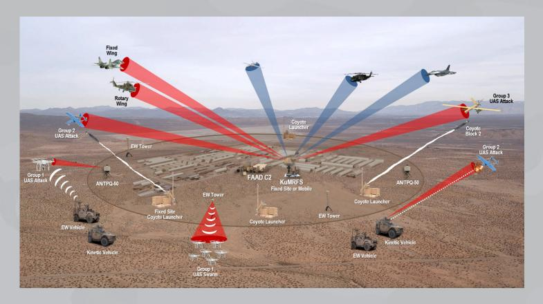
The Low, Slow, Small UAS Integrated Defeat System (LIDS) Family of Systems uses a range of passive and active sensors to detect, track and identify Groups 1 to 3 UAS and non-hostile aircraft. Using a comprehensive network to communicate, the command and control receives input from the sensors and allows the operator to task appropriate mitigation techniques in accordance with the Rules of Engagement, ranging from Electronic Warfare to full kinetic intercepts.
